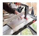
Spring-suspension individual plates support tiles while cutting
