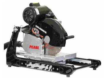
Model VX141MSPROD with 2 HP Induction Motor - 40% faster cutting and with greater power than any electric saw in its class! Size, Weight: 31.5" x 18.5" x 21", 110 lbs., 3250 RPM
