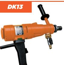
Hand held & portable. Side handle.14 amp. 580/1400/2900 RPM. Electronic overload. Dry Attachment. Thermal overload protection switch. Side handle for stability. Water connection for wet coring only. 5/8"-11 or 1.250"-7 Spindle. Three speed for bits up to 3" (6" mounted).
