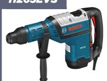
1-3/4" SDS-max® rotary hammer features best in class drilling & chiseling performance with 7.6 ft.-lbs. Impact energy (Penta). The hammer features 2 modes of operation. Rotary hammer or hammer-only & a variable speed dial for controlled drilling & chiseling applications. The tool also features the Vario-Lock™ function. This allows the chisel to be rotated into 12 different positions to optimize the working angle when used in hammer only mode.
