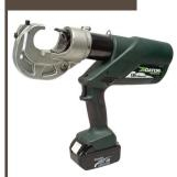
Intelligent Crimping System Technology includes a pressure sensor that monitors the crimping force of each crimp & provides the operator a visual & audible alert if the force is below specifications. State of the art 18V lithium ion (Li-ion) battery provides 70% more cycles per charge & faster cycle times. Automatic Retraction Stop (ARS) which retracts the ram just enough to get ready for the next cycle saving time & energy.
