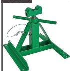
13"-27" Reel Stands. Wide, welded steel base for added stability with 5/8" holes. Roller bearings fit in the spindle groove to keep the spindle in place & turning freely. Two stands & a spindle are required for a complete setup.
