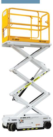
14' Electric scissor lift alternative to vertical mast lifts. Hy-Brid Lifts self-propelled series have high lifting capacities, low step-in heights & a lightweight design, making them the ideal choice for a variety of applications. Working height up to 20 ft. Weighs only 1650 lbs. Weight allows machine to go on delicate flooring. Lifts 670 lbs. Slide-out deck extension, with slip-resistant surface. Non-marking tires. Proportional controls. Full-Swing entrance door. Tilt alarm. Hour meter.
