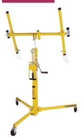
Drywall Lift w/ Hand Truck. Solid, safe construction. 2-speed winch handle. Quick, tool-free assembly. One person operation. Tilts 65deg. Lifts loads of 150Lb/70 Kg up to 11.5'/3.5m or 15'/4.5m. Loads at a convenient 34"/86 cm designed for safety.
