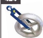
Hook Sheave 24". 4,000 lb. capacity. Forged steel hooks w/ 1 opening. Welded steel frames. 5" wide aluminum sheaves w/ self lubricating bearings.
