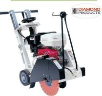
13hp Honda gas walk behind saw 18". 6-3/4" max cutting depth. Slip-on blade guards. Left or right side sawing. 18" max blade capacity. Cyclone air filter. Through rear axle for added strength. 3 V-belts for extra power delivery to the blade shaft. Solid, sealed self aligning blade shaft bearings.
