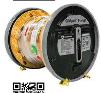
SIMpull Flange Cable Reel Feeder. Independently rotating flanges. Allows inner wooden reel to rotate freely. Shaftless design. Compatible with wooden reels up to 34" & 2000 lbs. 52lbs tare weight per Flange. Integral magnetic flange chocks. Will fit through 36" wide doorways when used with a 32" or smaller reel. Compatible with commercial & residential SIMpull® building wire products, parallels/stacks, portable cord, MV, & metal-clad cable.
