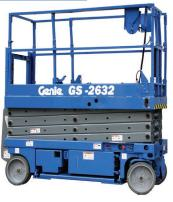
26' Scissor Lift. Zero-emission electric operation. 39" roll-out platform extension. High angle steering for excellent maneuverability. Folding rails with half-height swing gate standard on GS-2632. Universal 20 amp smart charger. Proportional controls for lift & drive functions. On-board diagnostics for easy troubleshooting. Multiple disc brakes provide smooth deceleration. Emergency stop at both platform& ground controls. Solid, non-marking tires. AC power to platform.
