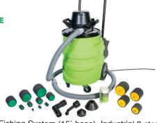
Power Fishing System (15' hose). Industrial 2-stage motor. Washable stainless steel filter. Fully equipped power fishing system. Large durable tank – large 12 gallon tank for wet or dry vacuum and storage for the available 15' hose. Air flow - Up to 107 cfm. Application - Powered conduit fishing.
