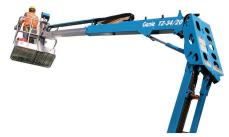
Articulating Z-Boom Lift 34' Trailer Mounted DC. Rugged & heavy-duty. Extension boom with self-leveling platform. Variable-speed control system. 359° non-continuous turntable rotation. Tilt alarm/sensor. Forklift pockets. Dual pneumatic jockey wheels for precise positioning during setup.
