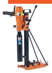
M-4 stand alone drill stand. Combination vacuum anchor angle stand for Weka motor, 30 long mast. Reversible slide handle. Quick release motor mount. High strength, hard anodized 1-5/8" x 2" aluminum column. Leveling bolts on all model bases. Hand held option. Carriage lock. 4 Leveling screws on base. Light weight & portable.
