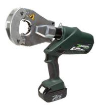
Intelligent Crimping System Technology includes a pressure sensor that monitors the crimping force of each crimp & provides the operator a visual & audible alert if the force is below specifications. State of the art 18V lithium ion (Li-ion) battery provides 70% more cycles per charge & faster cycle times. Automatic Retraction Stop (ARS) which retracts the ram just enough to get ready for the next cycle saving time & energy.
