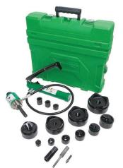
1/2"-4" Knockout Set. Compact design for field use on construction sites & maintenance jobs. Punches 10x faster than wrench method. Can be used w/ most standard round Slug-Buster® & Slug-Splitter SC® punches (not 1/2", 9/16", 5/8"). Can be used with non-round punches (adapter may be required). 3' hose. Powerful 11 ton hydraulic ram.
