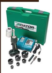
1/2"-2" Battery punch driver. Punch holes from any angle. 360° rotating head. Punches up to 6" holes in 14 gauge mild steel & 2" holes in 14 gauge stainless steel. Automatic retraction prevents damage to punch & die. One trigger controls all tool functions.
