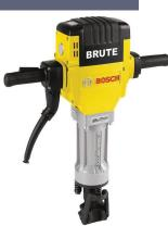
Brute Breaker Hammer. Total portability, operates on 115/120V AC/DC, 15AMP outlet or 2,500W portable generator. Vibration Control™ system, elongated air cushion in the hammer mechanism for all-day use. Ergonomic shock absorbing handles, also reduces vibration for greater user comfort. Service Minder™ brushes preventative-maintenance assurance for long tool life.
