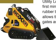
Boxer 32hp Kubota Diesel Compact Utility Loader with 44" bucket is the first mini-skid offering variable-width, rubber track undercarriage, which allows the units to enter through gates as narrow as three feet wide.
