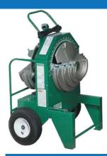
Features simple relay controls for easy field repairs & compact handle design to prevent interference with conduit when bending. The optional PVC-coated rigid conduit shoe group can be used on all 555 series benders. 20 AMP GFCI-Protected Receptacle VAC.
