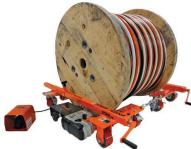
Jack up, transport, & power feed any wire (no lifting). Match speeds with iToolco Cannon 10K Puller. Light weight & wheeled for easy maneuvering. Adjustable size to any spool from 22" to 72" diameter. 5,000lb load capacity.
