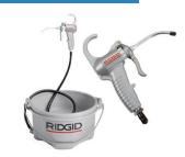
Pump assembly provides 50% more oil per stroke than other hand-held oilers for longer die life. An ergonomic 2-finger trigger design that reduces user fatigue. Die cast, heavy-duty body w/ swivel nozzle w/ no exposed parts for longer life. Features a patent pending fastener-less twist & lock drip pan that easily locks in place. The material withstands abrasion, is lighter than metal.
