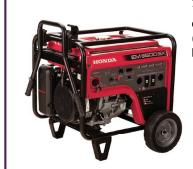
6500W, 120/240V. Provides 7,000W for 10 sec to start larger equipment. Powers fridge, freezer, furnace, well pump,& more. Long run time - up to 10.4 hrs. Powerful Honda iGX commercial engine. Electric start (battery included) with recoil back-up.
