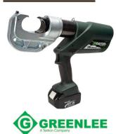
Intelligent Crimping System Technology includes a pressure sensor that monitors the crimping force of each crimp & provides the operator a visual & audible alert if the force is below specifications. State of the art 18V lithium ion (Li-ion) battery provides 70% more cycles per charge & faster cycle times. Automatic Retraction Stop (ARS) which retracts the ram just enough to get ready for the next cycle saving time & energy.
