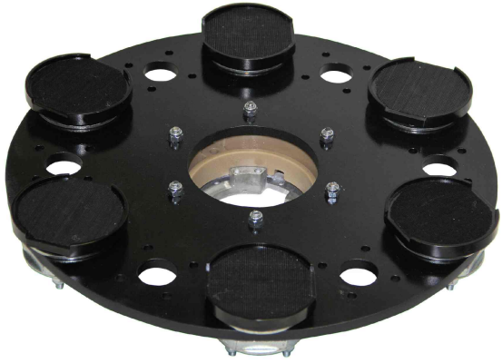
Orbitec Diamond Plate with (6) 3" Diamond Resin Pad Holders — Plate Spins Clockwise @ 175 RPM — — (6) Heads Spin Counter-Clockwise @ 400 RPM —
